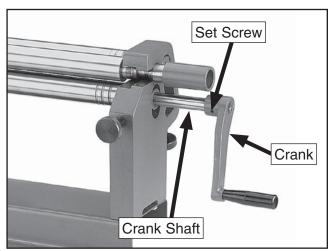
Figure 7. Crank mounting.
